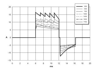
Figure A-6. Rectilinear Biphasic Waveforms at 50 Joules
