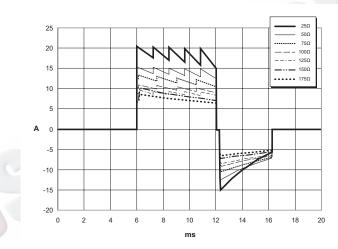
Figure A-5. Rectilinear Biphasic Waveforms at 70 Joules
