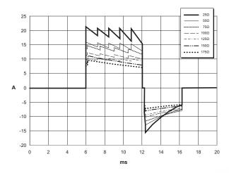
Figure A-4. Rectilinear Biphasic Waveforms at 85 Joules
