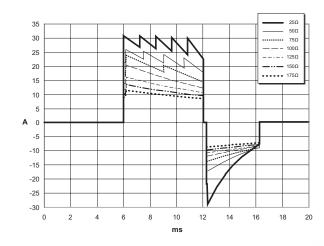
Figure A-1. Rectilinear Biphasic Waveforms at 200 Joules
