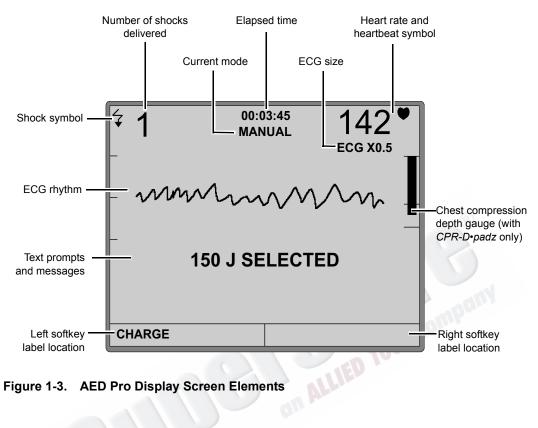
Figure 1-3 shows the layout of the screen and the location of the above items.
