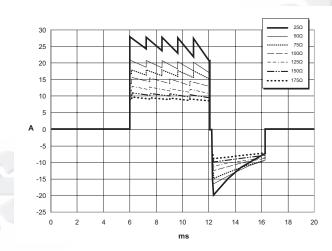
Figure A-2. Rectilinear Biphasic Waveforms at 150 Joules
