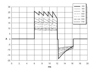
Figure A-3. Rectilinear Biphasic Waveforms at 120 Joules
